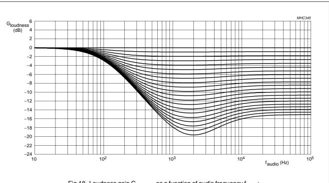
Fig.18 Loudness gain  $G_{loudness}$  as a function of audio frequency  $f_{audio}$ ; low boost frequency 100 Hz and high boost on.
